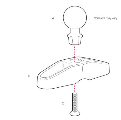
2 Connect castings to any vertical post using the hardware shown below.
